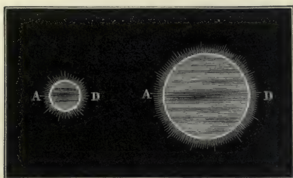
FIG. 64.—Images of planet produced by short and long focus lenses of the same aperture giving images of different size, but with the same amount of colour round the edges.
